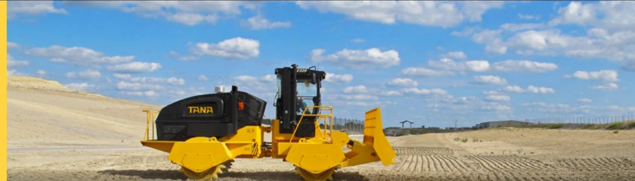
A TANA compactor's rigid frame maximizes the weight distribution of compaction into an area with uneven bumps.
