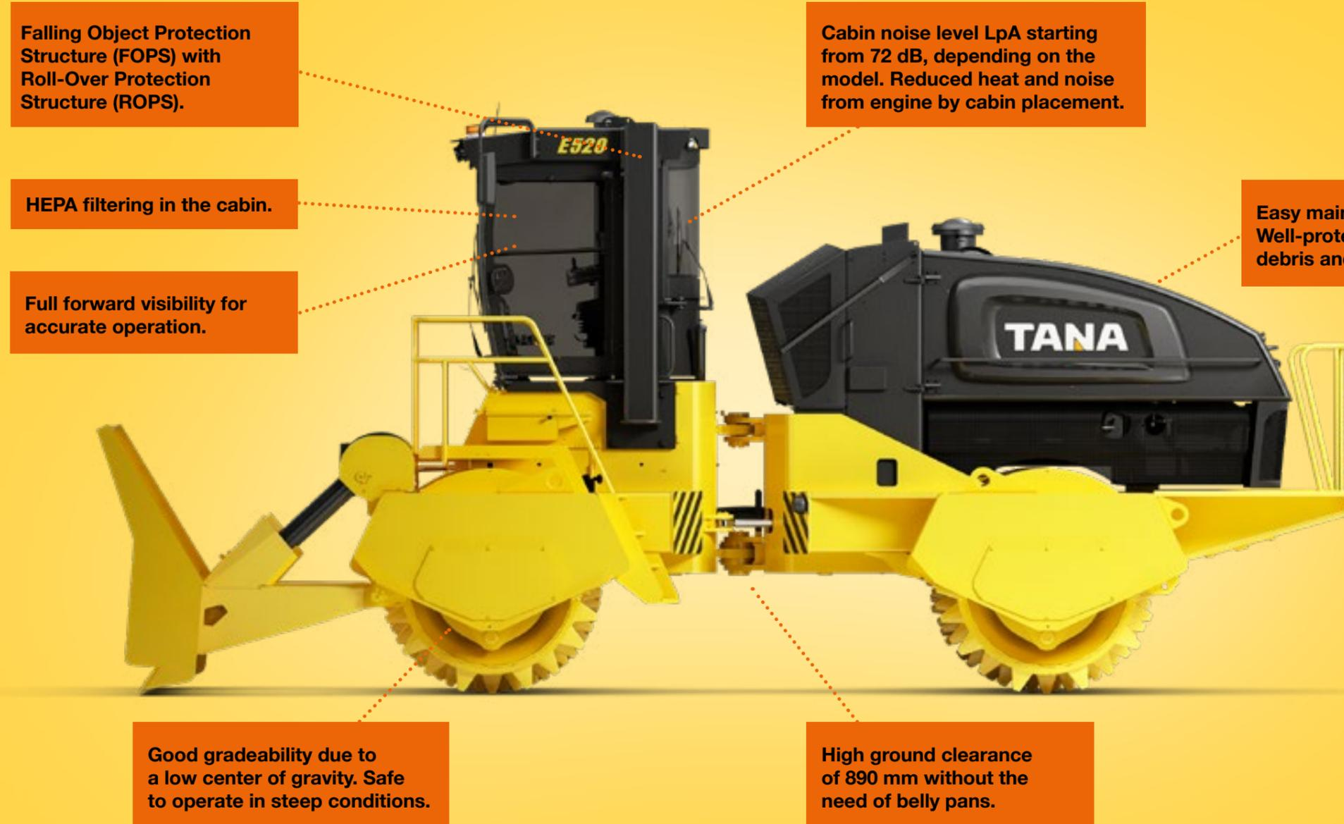
Falling Object Protection Structure (FOPS) with Roll-Over Protection Structure (ROPS).
