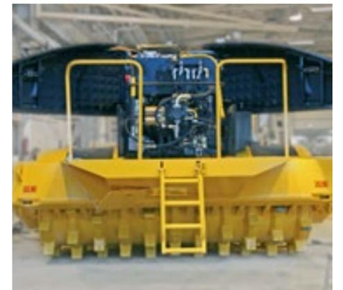
Simplicity in design provides a high uptime for TANA compactors. Easy access to the power pack from the rear saves time on routine maintenance operations and checkups. The optional ladders add usability for daily use.
