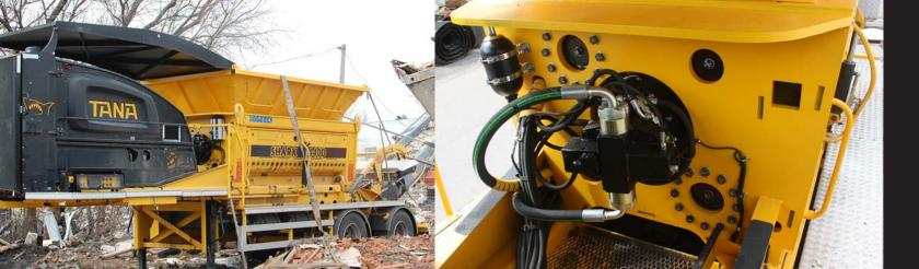
\*The swing frame construction (pat.) by TANA protects the gearbox, thus increasing reliability and maximizing uptime of the machine.
