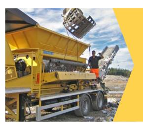
Adding or removing the rotor screen can be done in 10 minutes.
