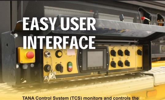
TANA Control System (TCS) monitors and controls the machine functions. There are 12 pre-programmed operating programs for different types of materials and purposes of shredding. On top of that, extra customer specified programs can be added.
