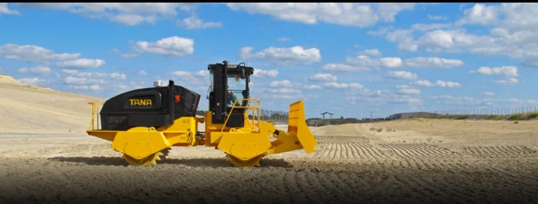
A TANA compactor's rigid frame maximizes the weight distribution of compaction into an area with uneven bumps.
